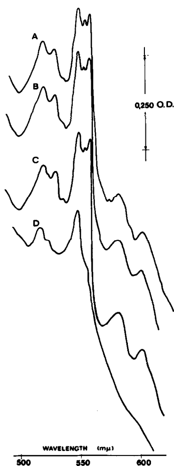
Fig. 1 - Low-temperature spectra. The spectra of cytochromes reduced by sodium dithionite were obtained at -190^{\circ} with a Cary 14 Spectrophotometer specially equipped (11). 0.5 ml of a suspension of 1 \times 10^{10} cell/ml was used for each spectra. A: wild-type S. cerevisiae grown at 23^{\circ} ; B: wild-type at 36^{\circ} , grown with galactose as carbon source; C: 1511 mutant grown at 23^{\circ} , and D: some mutants grown at 36^{\circ} with galactose.
